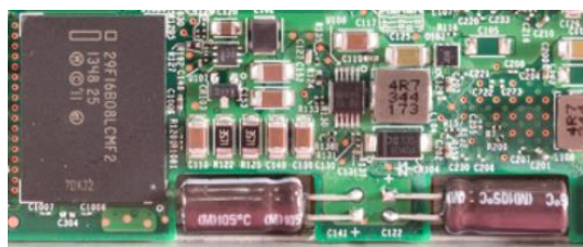
Figure 2: Tantalum Capacitors for Cache Flushing
